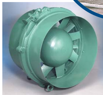
8 1524 0300 Pneumatic Axial Fan, 24" dia. 12,353 cfm output @ 90 psi
